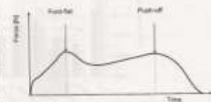
FIGURE 2. Ground reaction force during the whole foot-floor contact. The first peak corresponds to foot-flat and the second one to push-off.
